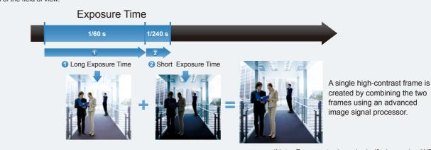
(Note: Frame rate drops by half when using WDR Pro.)
