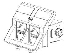
Can: 0.25mm brass to C2680R preplated tin over nickel IDC Connector Plastic Housing: Polycarbonate, UL94V-0 rated or equivalent Operating Life: Min. 20 Reterminations Contact Material: Copper Alloy IDC Contact Plating: Tin/Lead Plate Contact Force: 100g minimum Wire Accommodation: 22-24 AWG solid
