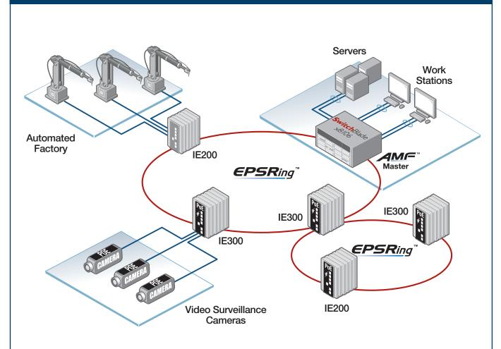
EPSRing<sup>™</sup> ITU-T G.8032 provide high speed resilient ring connectivity; this diagram shows the IE Series in a double ring network topology.
