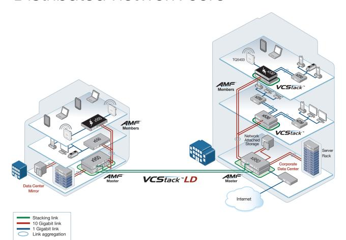
Today's corporate network users demand a high-performing enterprise network that can seamlessly carry multiple converged services, and provide instant access to online resources and applications. This key solution uses the x950 Series and VCStack LD—ideal for a distributed business network core that provides high availability, increased capacity and ease of management.
